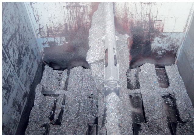
Figure 1: Fully automatic sampling at RDF unloading station; Photo: MVW Lechtenberg
